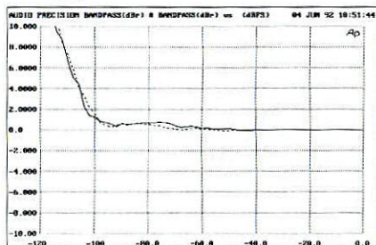
Fig.10 CAL System I, MASH IV DAC departure from linearity (right channel dashed, 2dB/vertical div.).
