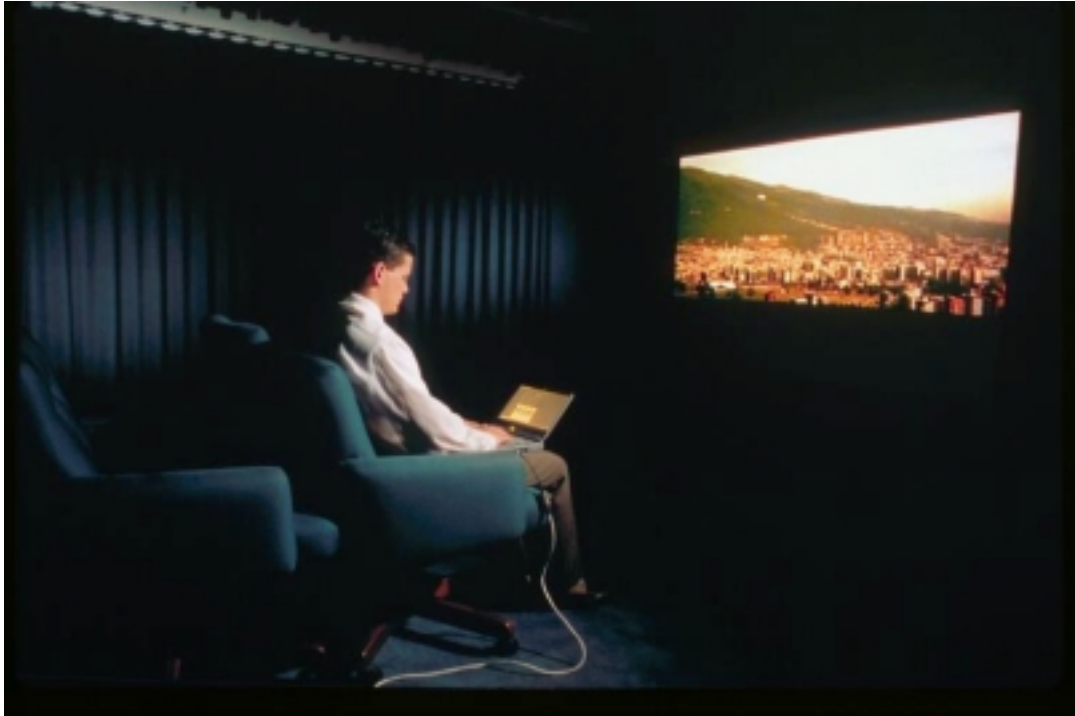
Figure 6 A listener performing a test by entering their data on a laptop computer that is networked to the NT Server. In this test, video is displayed and both front, side and rear curtains are drawn to hide the identifies of the 5.1 loudspeaker systems under test.
