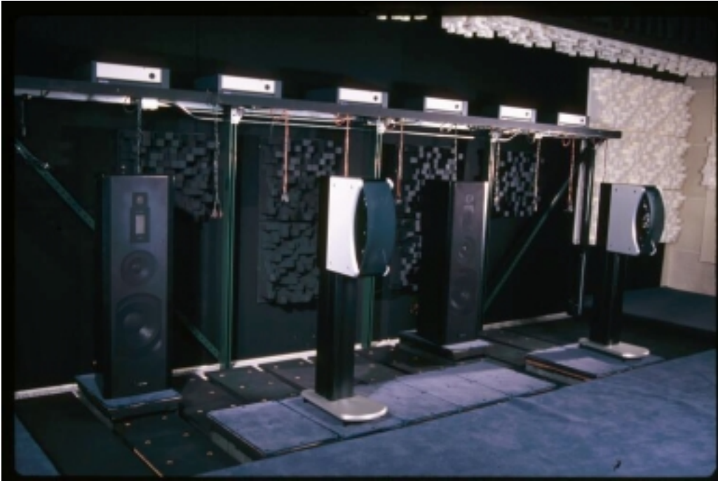
Figure 4 Shown is the automated speaker shuffler of the MLL set up for A/B stereo testing of two stereo loudspeakers. Here the front listening screen is pulled up.
