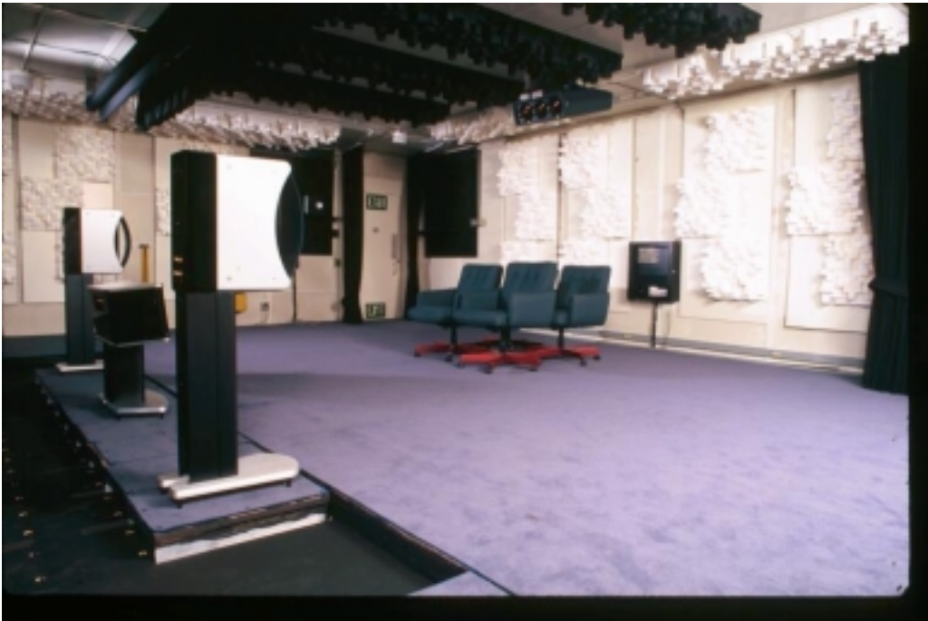
Figure 5 A front-left wide-angle shot of the MLL with the listening screens pulled back. The automated speaker shuffler is in the foreground setup for 5.1 playback. Note the side and rear channel speaker baffles in the background, and the audio and computer data control box on the back wall. The video projector is mounted on the ceiling with a retractable screen in front of the speaker mover.
