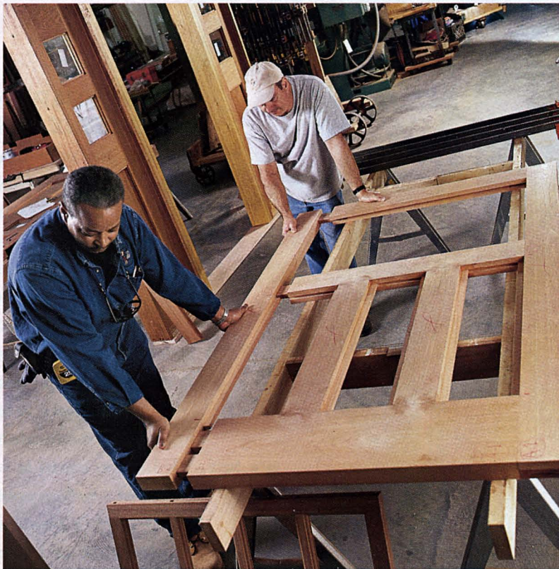
Door makers at Hahn's Woodworking Company fit together the stiles and rails of a panel door. Mortise-and-tenon joinery is the most common method used on custom doors, because of its strength and durability.
